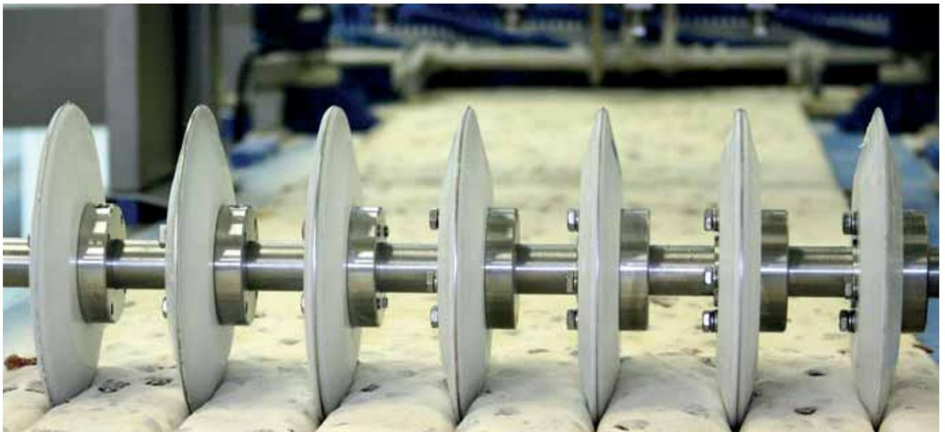
Cutting a sheet of dough on Rademaker's Crusto bread line.
